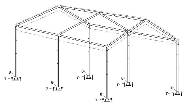
Figure 7: Foot Plate (8) Assembly
